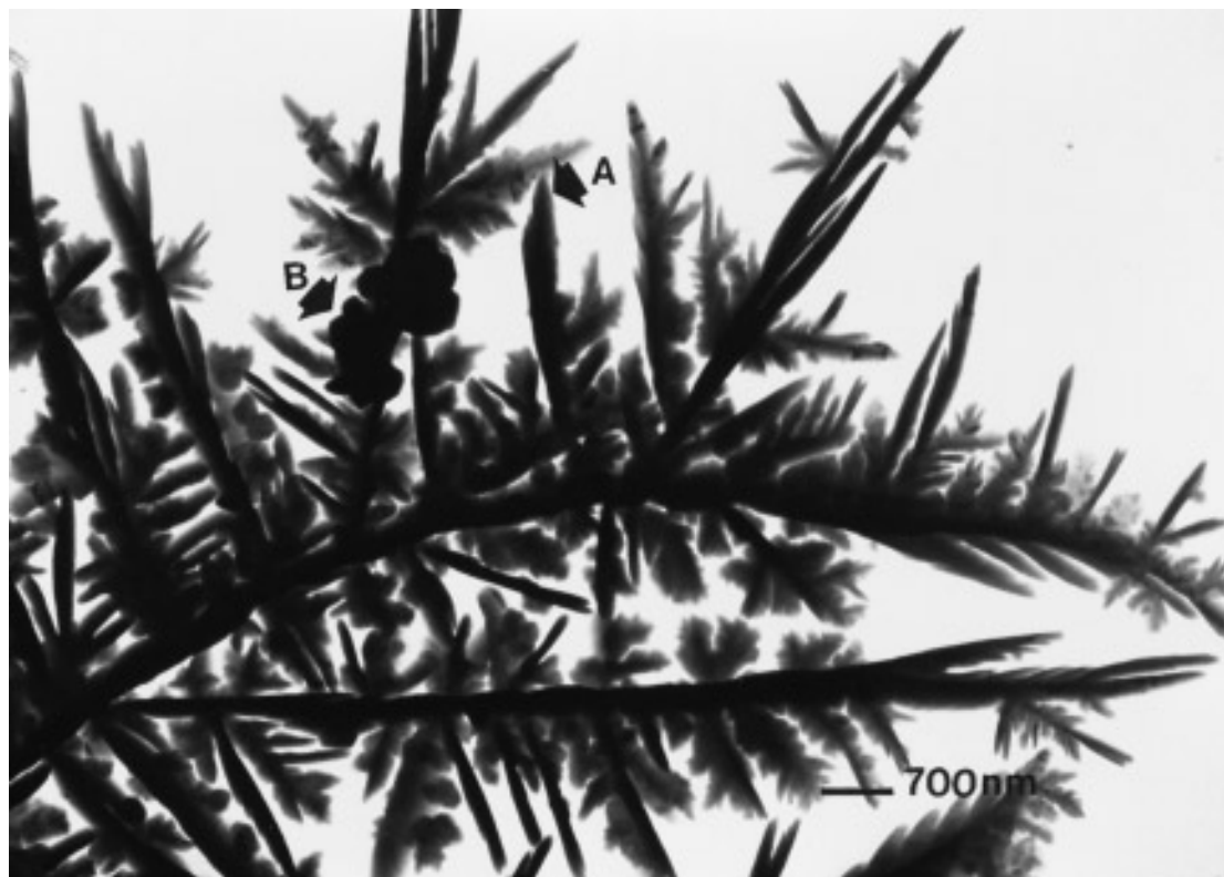
FIG. 7. Typical micrograph of T-NiW-F(x) catalysts showing a tree-like phase (A) and another phase (B) which resembles (\text{NH}_4)_2\text{WS}_4 crystallites attached to phase (A).
